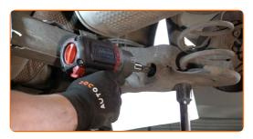
Remove the fastening bolt.
