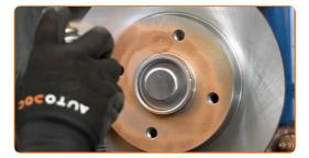
Clean the brake disk surface. Use all-purpose cleaning spray.
