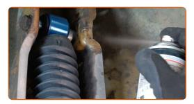
Tighten the lower fastener of the shock absorber. Use a drive socket #E16. Use a torque wrench. Tighten it to 100 Nm torque.
