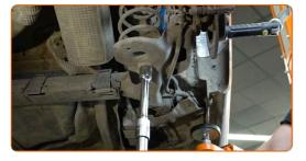
Tighten the top shock absorber fastening. Use a drive socket #16. Use a torque wrench. Tighten it to 60 Nm torque.
