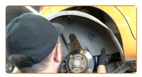
Reinstall the plastic clips of the wheel arch liner.
