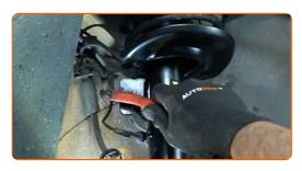
Install a new rod, tighten the fasteners.
