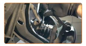
Unscrew the fastener connecting the stabilizer link to the shock strut. Use a combination spanner #16. Use Torx T30. Use a ratchet wrench.
