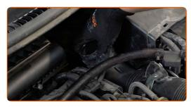
Remove the air intake pipe.
