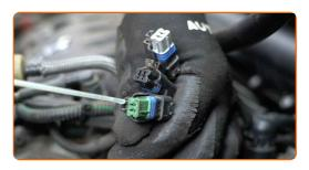
Attach the engine wiring harness connectors.
