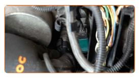
Install the engine wiring harness cover. Make sure you hear a click indicating that it is locked in place.
