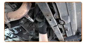
Drain the coolant from the engine.
