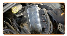
11 Remove the engine wiring harness cover.
