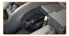
Disconnect the charger intake hose from the air filter housing.
