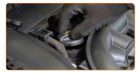
Pour oil into the engine through the filler. Required amount of oil: 4.25 l.
