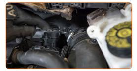
16 Install the brake fluid reservoir.
