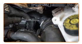
6 Undo the fastening screws of the air filter cover (3 pieces). Use Torx T25. Use a ratchet wrench.
