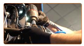
Disconnect the tie rod end from the steering knuckle. Use a pin punch. Use a hammer.
