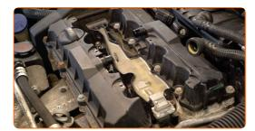
Tighten the fasteners of the ignition coils. Use Torx T20. Use a torque wrench. Tighten it to 8 nm torque.
