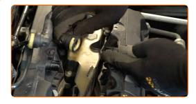
6 Detach the connector from the ignition coil.
