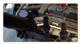
Plug in the ignition coil connector.
