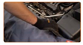
Unscrew the engine cover fastener. Use Torx T20.
