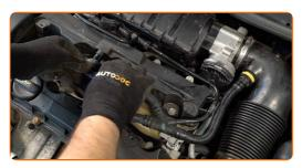
Install the engine cover and secure it. Screw in the engine cover fasteners. Use Torx T20.
