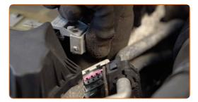
Unscrew the ignition coil bracket. Use Torx T27.
