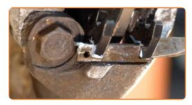
15 Install the brake pad retaining pin.
