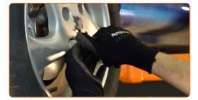
Lower the car and working in a cross order, tighten the wheel bolts. Use a torque wrench. Tighten it to 100 Nm torque.
