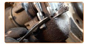
Remove the brake pads. Use a crowbar.
