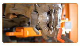
Remove the retainer of the brake pads. Use a crowbar. Use a rubber mallet.
