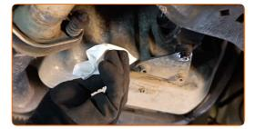
Screw in the new drainage plug and tighten it. Use a drive socket #24. Use a torque wrench. Tighten it to 30 Nm torque.
