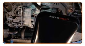
6 Unscrew the drain plug. Use a drive socket #24.
