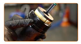
Screw the new filter into its place.
