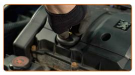
Tighten the oil filler cap.
