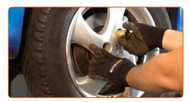
Lower the car and working in a cross order, tighten the wheel bolts. Use wheel impact socket #19. Use a torque wrench. Tighten it to 100 Nm torque.
