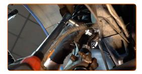
Tighten the fastener connecting the stabilizer link to the stabilizer bar. Use a combination spanner #17. Use Torx T30. Use a torque wrench. Tighten it to 35 Nm torque.
