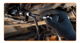
Unscrew the fastener connecting the stabilizer link to the shock strut. Use a combination spanner #17. Use Torx T30. Use a ratchet wrench.
