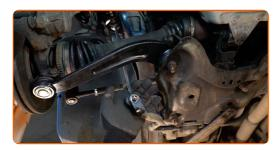
Tighten the fastener connecting the stabilizer link to the shock strut. Use a combination spanner #17. Use Torx T30. Use a torque wrench. Tighten it to 35 Nm torque.
