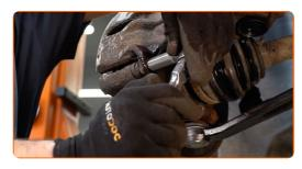
10 Remove the brake caliper.
