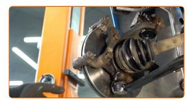
Tighten the brake caliper bracket. Use a drive socket #19. Use a torque wrench. Tighten it to 105 Nm torque.
