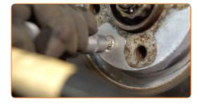
16 Remove the brake disc.
