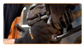
10 Remove the brake caliper.
