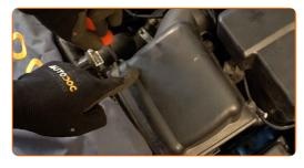
Remove the fender protection cover.
