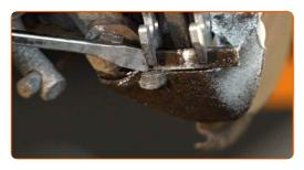
10 Remove the brake pads. Use a crowbar.
