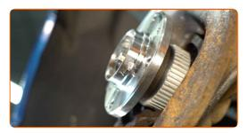
Tighten the hub. Use a drive socket #32. Use a torque wrench. Tighten it to 230 Nm torque.
