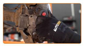
Remove the brake caliper.
