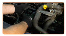
Attach the fuel pressure sensor connector.
