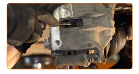
Remove the brake caliper.
