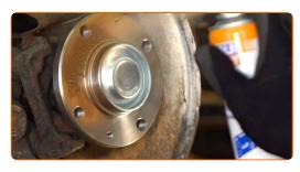
Install the brake disc.
