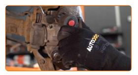
13 Remove the brake caliper.
