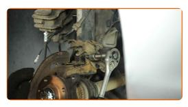
Connect the ABS sensor wiring.
