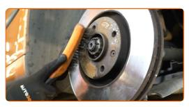
Unscrew the brake disc fasteners. Use a Phillips screwdriver.
