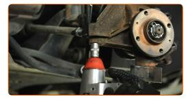
Install the bracket on the suspension strut.
