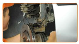
Unscrew the ABS sensor wiring bracket. Use a drive socket #10. Use a ratchet wrench.
