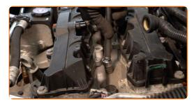
Screw new spark plugs and tighten them. Use the spark plug socket #16. Use a torque wrench. Tighten it to 26 nm torque.
