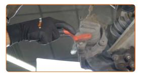
8 Unscrew the brake caliper fastening. Use a combination spanner #13.
