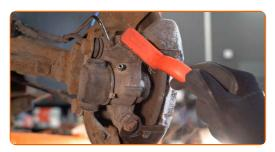
Unscrew the brake caliper fastening. Use a drive socket #19. Use a ratchet wrench.
