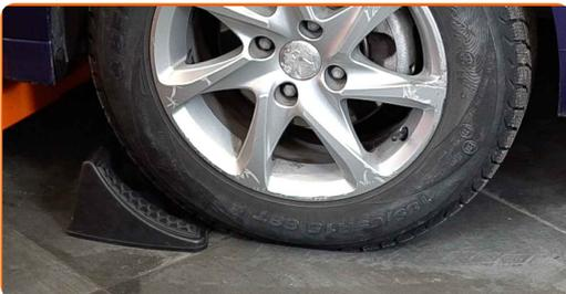
**5** Loosen the wheel mounting bolts. Use wheel impact socket #17.
