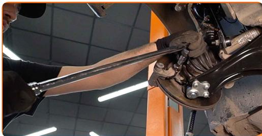
**16** Remove the caliper bracket.
