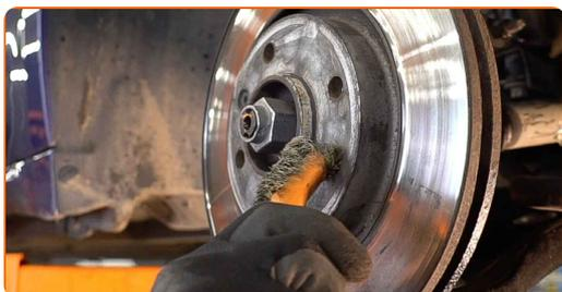
**18** Unscrew the brake disc fastening. Use Torx T30. Use an impact screwdriver.
