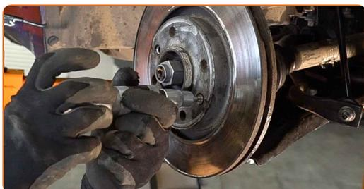
19 Remove the brake disc. Use a rubber mallet.
