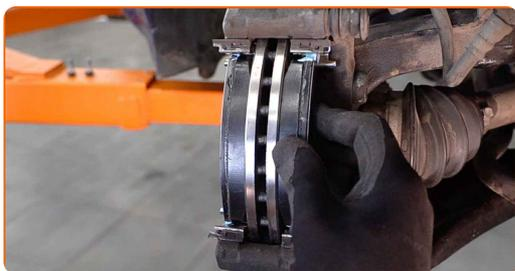
**29** Install the brake caliper and fix it. Use a combination spanner #13. Use a drive socket #13. Use a torque wrench. Tighten it to 30 Nm torque.
