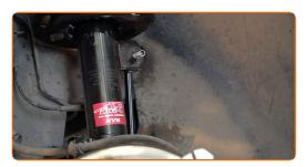
Tighten the fastener connecting the stabilizer link to the stabilizer bar. Use a drive socket #16. Use a torque wrench. Tighten it to 43 Nm torque.
