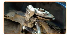
Tighten the top shock absorber fastening. Use a combination spanner #19. Use a drive socket #19. Use a torque wrench. Tighten it to 70 Nm torque.
