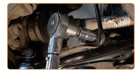
Tighten the fastener connecting the stabilizer link to the shock strut. Use a drive socket #16. Use a torque wrench. Tighten it to 43 Nm torque.
