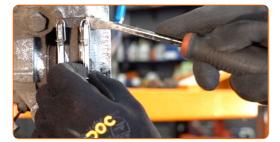
Remove the brake pad retaining pin. Use round-nose pliers.
