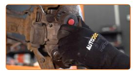
13 Remove the brake caliper.
