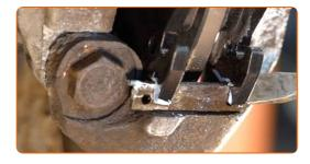
Install the brake pad retaining pin.
