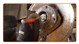
Unscrew the wheel hub axle nut. Use a drive socket #32. Use a tap wrench.
