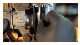
Install the retainer of the brake pads. Use a crowbar.
