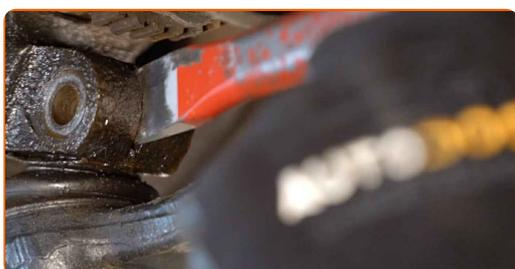
**16** Prop up the steering knuckle. Use a hydraulic transmission jack.
