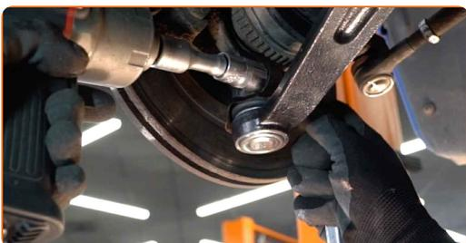
**34** Tighten the front fastener connecting the control arm to the subframe. Use a drive socket #21. Use a torque wrench. Tighten it to 111 Nm torque.
