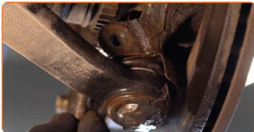
**15** Release the fastener that connects the control arm ball joint to the steering knuckle. Use a flat metal-working chisel. Use a hammer.
