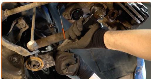
25 Clean the mounting seats and the thread of the suspension arm. Use a wire brush. Use WD-40 spray.
