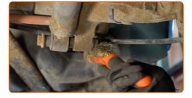
Unscrew the upper fastener of the shock absorber. Use a combination spanner #19. Use a drive socket #19. Use a ratchet wrench.
