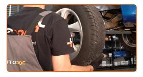
Clean the shock absorber fasteners. Use a wire brush. Use WD-40 spray.
