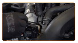
3.2 Squeeze the clamp with combination pliers and disconnect the vacuum valve hose.
