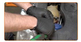
Remove the coolant reservoir cap.
