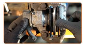
Replacement: brake pads – PEUGEOT 206 Hatchback (2A/C). Tip:
