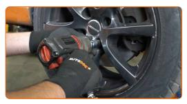
Lower the car and working in a cross order, tighten the wheel bolts. Use wheel impact socket #17. Use a torque wrench. Tighten it to 100 Nm torque.
