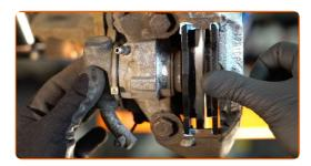
Install the retainer of the brake pads. Use a crowbar.
