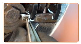
27 Install the retaining springs of the brake pads.
