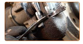
Remove the brake pads. Use a crowbar.
