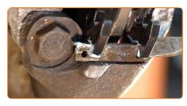
26 Install the brake pad retaining pin.
