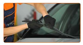
Remove the blade from the wiper arm.
