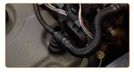
Remove the crankcase ventilation hoses.
