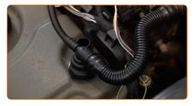
Remove the crankcase ventilation hoses.
