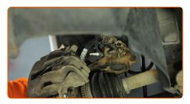
Remove the brake caliper together with its bracket.
