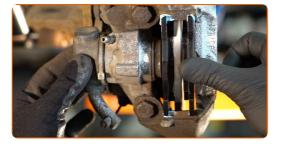
Replacement: brake pads – PEUGEOT 205 I Hatchback. Tip:
