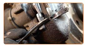
Remove the brake pads. Use a crowbar.
