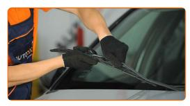
Remove the blade from the wiper arm.
