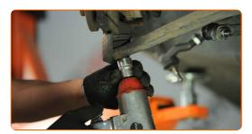
Disconnect the lower control arm from the steering knuckle. Use a ball joint puller. Use a crowbar.
