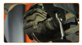
Connect the brake pad wear sensor plug.
