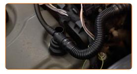
Remove the crankcase ventilation hoses.
