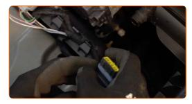
Detach the connector from the ignition coil.
