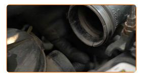
6 Release the air filter cover clips.
