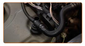
Remove the crankcase ventilation hoses.
