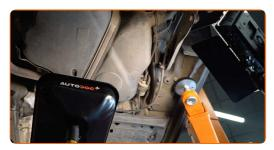
Unscrew the drain plug. Use a combination spanner #22.
