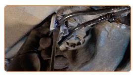
Squeeze the clips and detach the fuel supply lines from the fuel filter housing. Use fuel line pliers. Use a crowbar.
