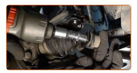
Unscrew the fastener connecting the stabilizer link to the shock strut. Use a drive socket #16.
