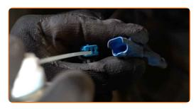
Attach the ABS sensor connector.
