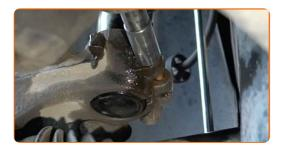
Remove the fastening bolt.
