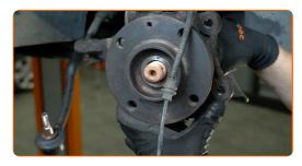
63 Attach the ball joint to the control arm.
