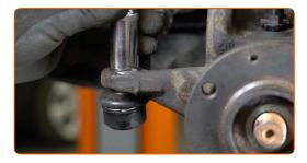
Tighten the fasteners connecting the ball joint to the control arm. Use a drive socket #16. Use a torque wrench. Tighten it to 60 Nm torque.
