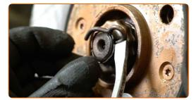
Loosen the fastener of the driveshaft. Use a drive socket #35. Use a tap wrench.
