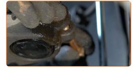
Detach the driveshaft from the steering knuckle.
