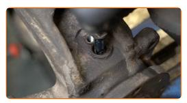
Tighten the fastener that connects the ABS sensor to the steering knuckle. Use a drive socket #13. Use a torque wrench. Tighten it to 10 nm torque.
