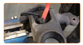
Unscrew the ABS sensor fastener. Use a drive socket #13. Use a ratchet wrench.
