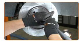
24 Remove the brake disc.
