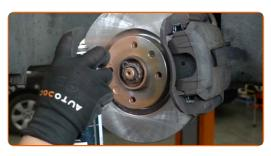
Olean the brake disk surface. Use a brake cleaner.
