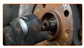
Clean the stabiliser link fasteners. Use a wire brush. Use WD-40 spray.
