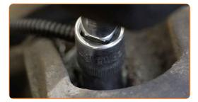
Disconnect the ABS sensor. Use a flat screwdriver.
