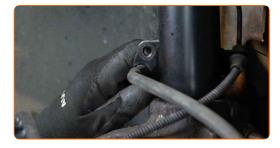
Tighten the fastener connecting the brake hose bracket to the suspension strut. Use a drive socket #13. Use a torque wrench. Tighten it to 10 nm torque.
