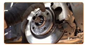
Detach the driveshaft from the steering knuckle.
