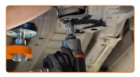
13 Remove the fastening bolt.
