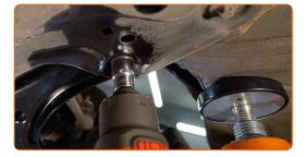
Screw the front arm fastener. Use a drive socket #18.
