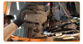
Connect the ball joint to the steering knuckle. Use a crowbar.
