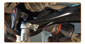
Screw the rear arm fastener. Use a drive socket #18.
