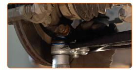
Screw the fastener connecting the ball joint to the steering knuckle. Use a drive socket #16. Use a drive socket #E8. Use a ratchet wrench.
