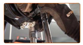
Tighten the front fastener connecting the control arm to the subframe. Use a drive socket #18. Use a torque wrench. Tighten it to 120 Nm torque.
