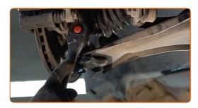
9 Remove the fastening bolt.
