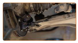
Loosen the rear fastener of the control arm. Use a drive socket #18. Use a tap wrench.
