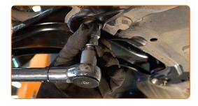
Tighten the rear fastener of the control arm. Use a drive socket #18. Use a torque wrench. Tighten it to 120 Nm torque.
