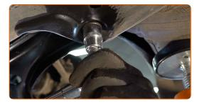
Remove the support from under the arm.
