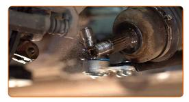
Mount the drive shaft into the wheel hub.
