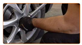
Tighten the wheel bolts using a criss-cross pattern. Use a torque wrench. Tighten it to 100 Nm torque.
