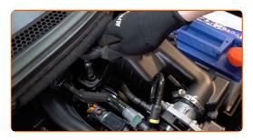
6 Disconnect the air intake pipe from the air filter housing.
