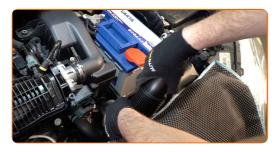
Remove the air filter housing.
