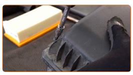
Reinstall the air filter housing.
