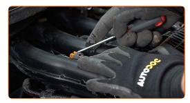
Unscrew the ignition coil bracket. Use a drive socket #8.
