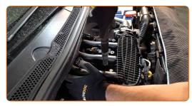
7 Unscrew the spark plugs. Use the spark plug socket #16.
